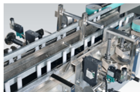
Hot melt sealing
